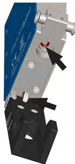
Piezo actuator cleaning locations (do not use sharp tools)
