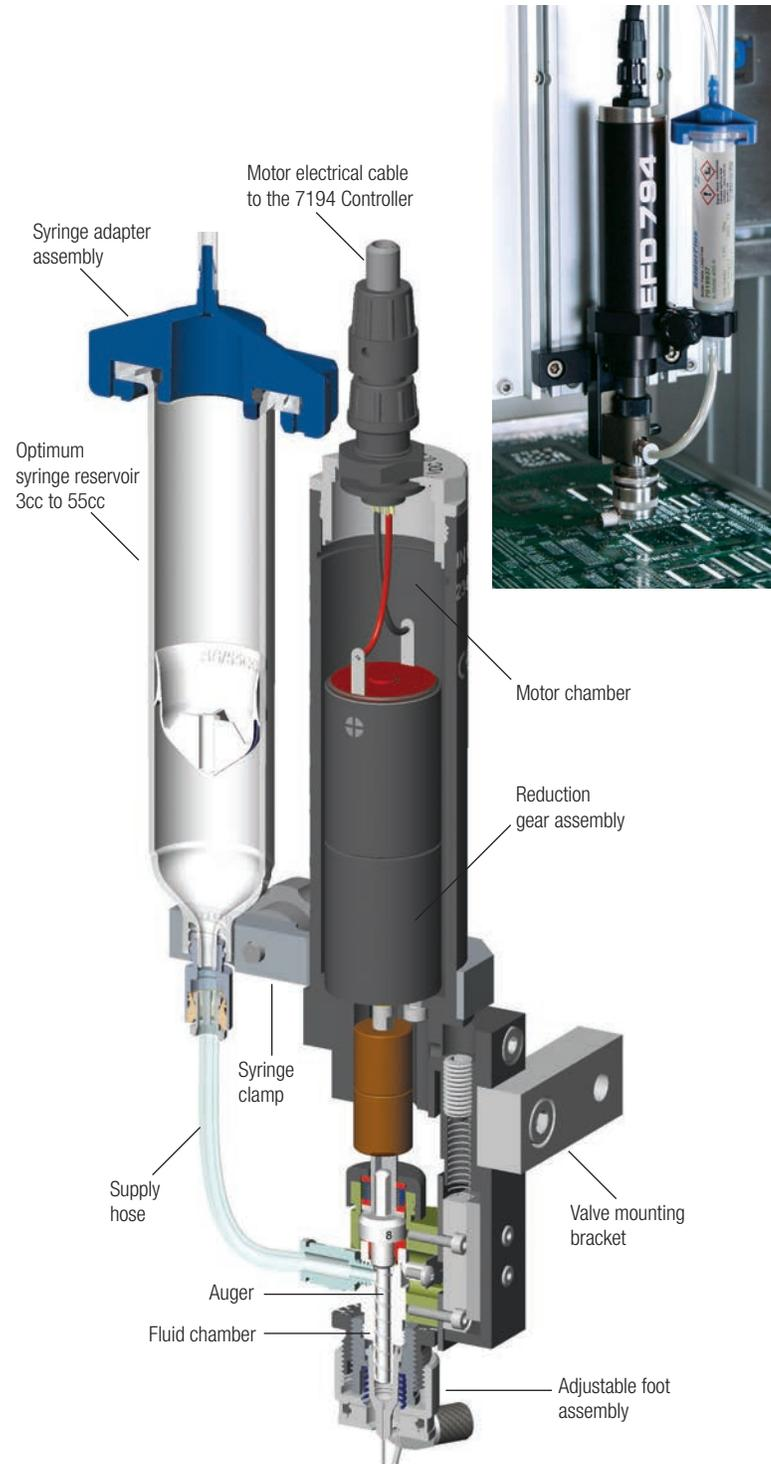
The 794 Series auger valve system is designed to make precise, repeatable deposits of solder paste. By integrating screw feed technology with precise control of dispense time, syringe pressure, and auger speed, the 794 Series system ensures consistent deposits without damage to the metal alloy particles in the solder paste.
