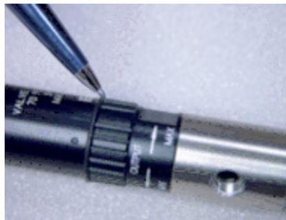
2. Install the 1/8 NPT rod in the fluid body mounting hole or fluid inlet.
