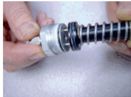
4. Install the air cylinder cap, piston and spring by pushing to compress the spring while turning to engage the threads.
