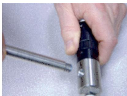
3. Holding the rod, use an 8" adjustable wrench to remove the fluid body cap.
