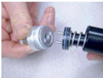
The valve is now completely disassembled, and is ready for cleaning, inspection and reassembly.
