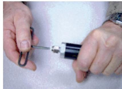
**9. Install the fluid body and tighten using the 1/8 NPT rod and 8" adjustable wrench. If a torque wrench is available, torque to 6.78 Nm (5 ft lbs).**
