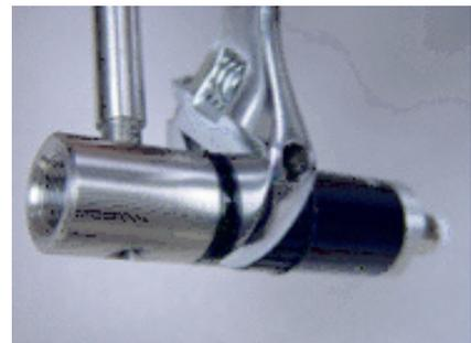
**10. Install the sealing head and screw using the 1/4" flat tip screwdriver. If a torque screwdriver is available, proper torque is 1.69 nm (15 in lbs).**
