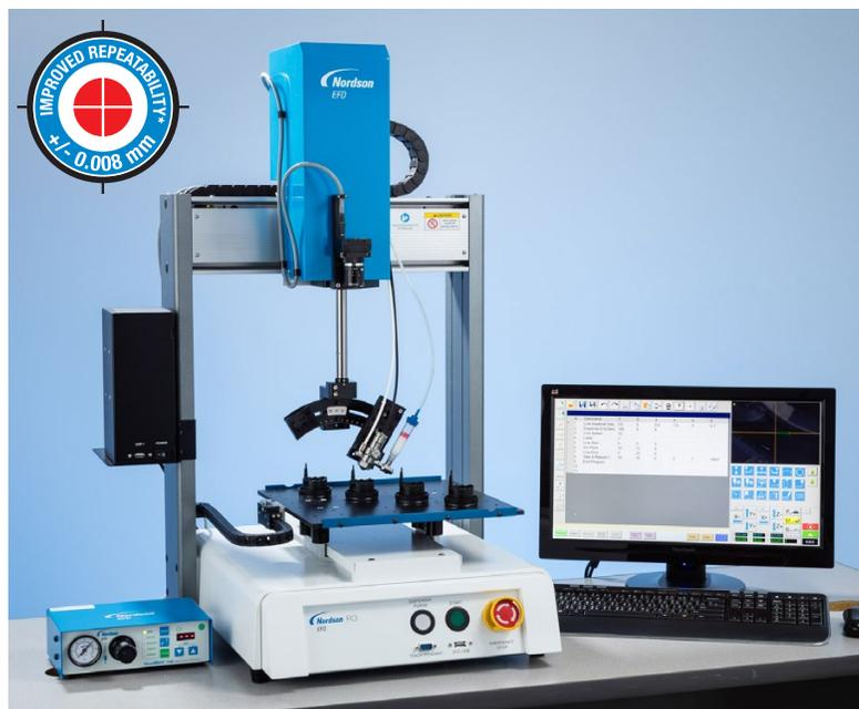
RV Series makes 4-axis dispensing automation more intuitive with proprietary DispenseMotion software.
