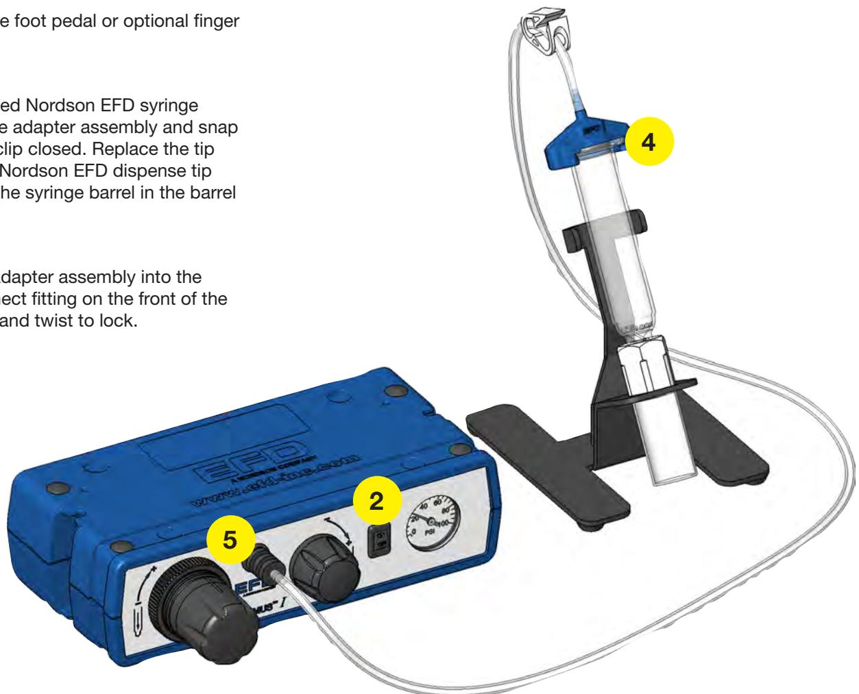
6. Unsnap the safety clip. Depress and hold the foot pedal for the remainder of this setup.
