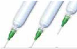
**Remember** - always bring the tip in contact with the work surface at the illustrated angle. After the tip is in position, press the foot pedal. Release pedal and remove tip by lifting straight up.
